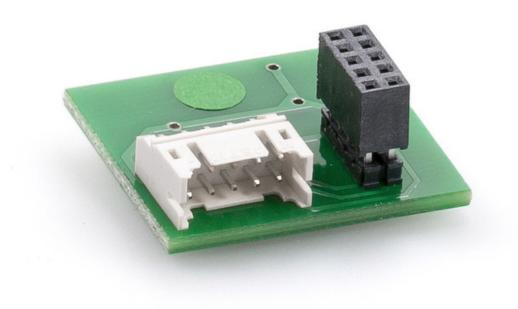
Insertable interface board for series connection of a maximum of two self-monitoring GC 363 SF combined detectors
