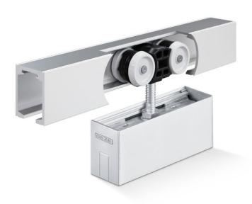
Sliding door fitting system for glass doors with a leaf weight of 80 kg and fixed panel and a 30 mm glass clamping plate attached to the ceiling
